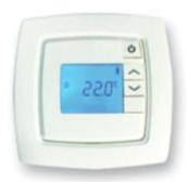
An active room sensor will help the heat pump to adjust the supply line temperature in situations where the indoor temperature changes as a result of unmonitored heat sources, such as separate firewood place or high solar radiation.
